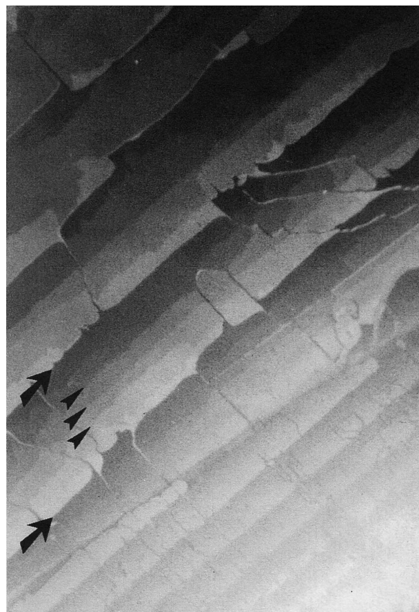
Figure 20. Optical microphotograph of a TGB C sample in a wedge with planar anchoring between crossed polarisers. A \lambda/4 plate is inserted. The photograph size is 220 \times 330 \mu\text{m}^2 . The TGB C phase coexists with the cholesteric phase visible in the south-east corner. A series of parallel lines (small arrows) appears in the TGB C phase only, in between the usual Grandjean–Cano steps (large arrows). These new defects are interpreted as edge dislocations of the layered array of smectic slabs forming the TGB structure (from (49)).
